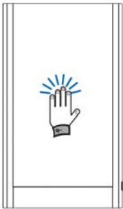
Front pad will not illuminate when batteries are exhausted
